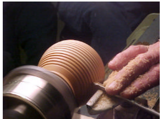
Cutting grooves on lidded box
